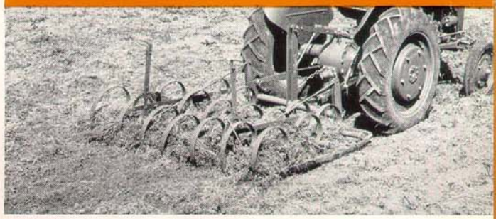
1 Lifting of harrow sections by hand to clear them of trash is eliminated by the Ferguson System.
