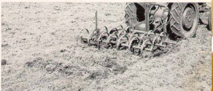
3 With the teeth clear, another touch on the hydraulic control lowers the harrow to working depth, all without effort and without stopping the tractor.
