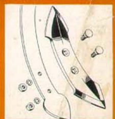
Above—This drawbar and a third section quickly converts a two-section harrow to three sections.
