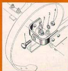
Left—Lock-type clamp which secures the teeth to the tooth bars.
