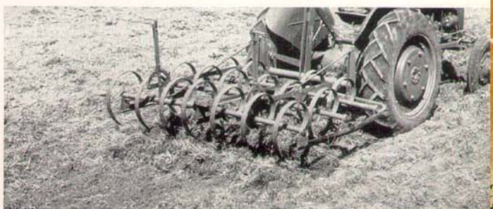
2 If the harrow clogs, a finger tip touch on the hydraulic control raises all sections without stopping the tractor, to drop or spread the trash, as desired.
